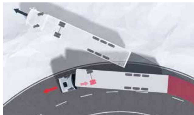
ESP compensatory braking when vehicle is understeered
