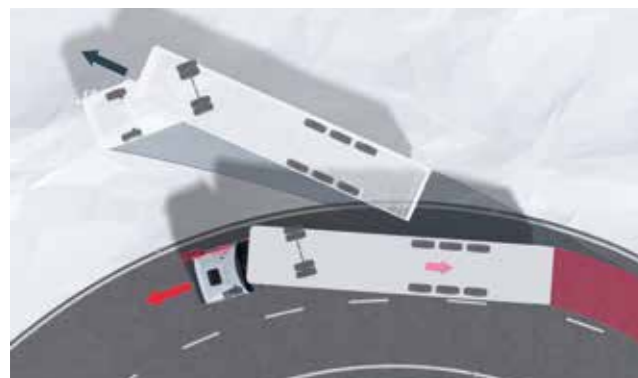
ESP compensatory braking when vehicle is oversteered
