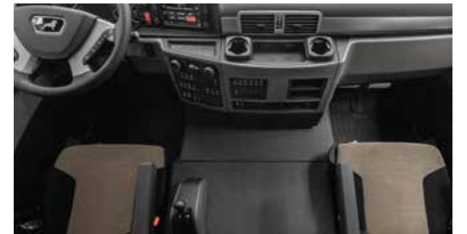
Rearranging the TipMatic switch and parking brake creates additional space
